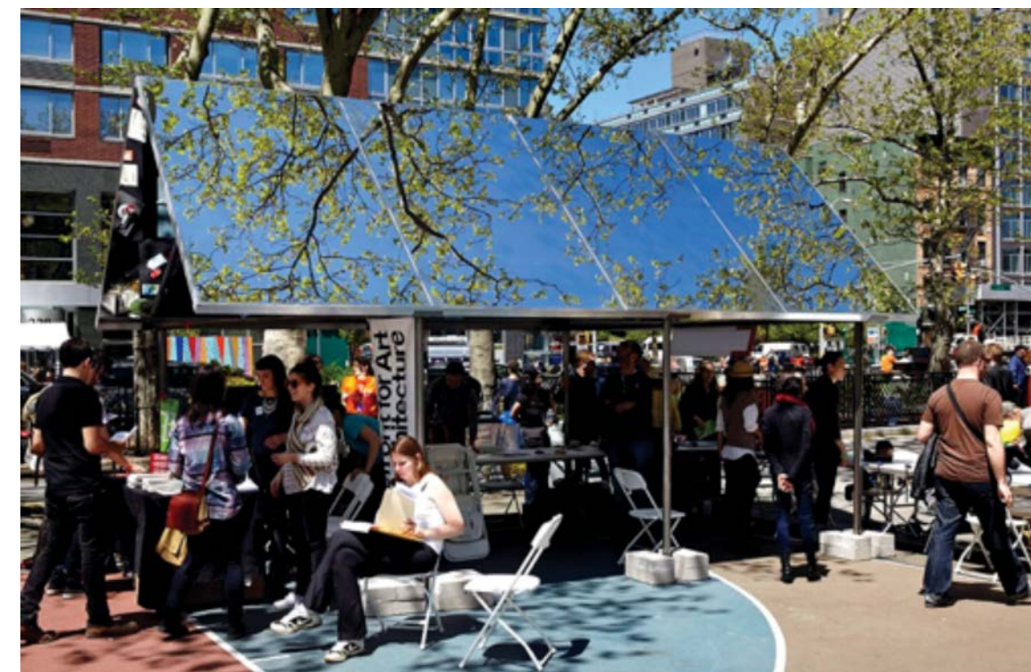
RIGHT MirrorMirror's design includes a simple forty-five-degree-angled gable roof made from mirroring panels. When combined, the units create a large barn-like structure for hosting gatherings within. Photo by Benoit Pailley
